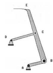
Crank AB drives the motion. The hook at E is required to advance the film downward, with engagement and disengagement close to right angles to the film. The linkages have tolerance of 0.01 on their lengths and 0.1 on their angles. We will design such a mechanism and verify that the mechanism indeed produces a downward motion that satisfies the engagement and disengagement requirements.
