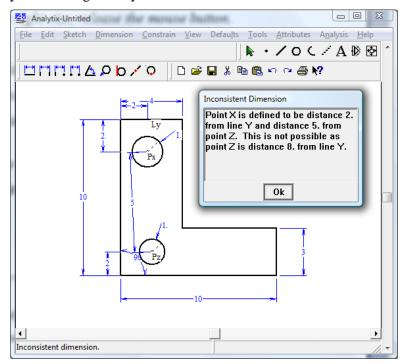
The message tells you the reason for the problem: that the center of G is distance 5 from the center of H and only 2 from line BC, but line BC is distance 8 from the center of circle H. The problem can be resolved if the distance from circle centers G to H is changed to 6.
