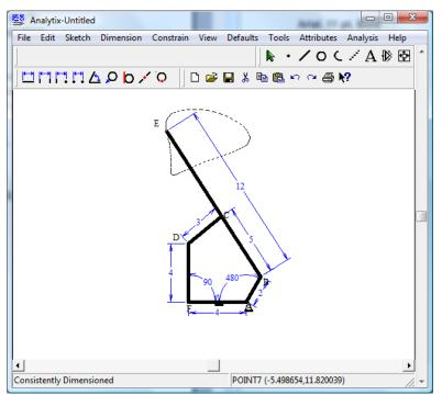
The trace of point E's motion appears with a cuspid like shape. The trace confirms that point E moves downward in a straight line and its engagement and disengagement movements do occur at close to right angles.
