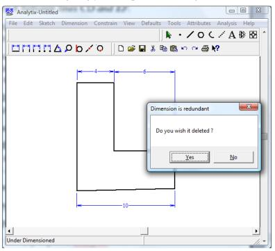
The dimension is redundant because the distance between CD and EF is already defined as a result of the distance between lines AB and EF and the distance between lines AB and CD.
