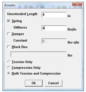
Enter "4" in the Unextended length field Click on the Spring box to select it Enter the spring constant "10 "in the Stiffness field
