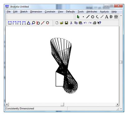
Analytix displays the envelope of the geometry's motion as line AB cranks over the full revolution. Notice that line BE's envelope follows the trace of point E.
