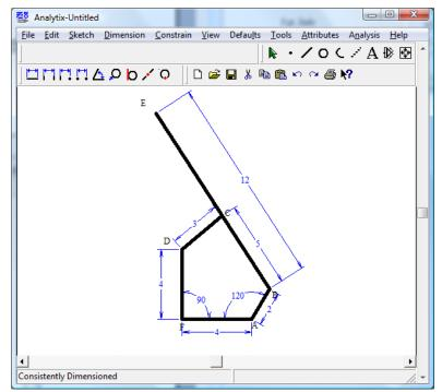
To fully dimension the geometry, we will set angle BAF to 120. This is the driving angle for the mechanism. Once angle BAF has been specified, the geometry is consistently dimensioned as evidenced by the "Consistently Dimensioned" message in the Dimension Status Box and Analytix draws the geometry to scale automatically.
